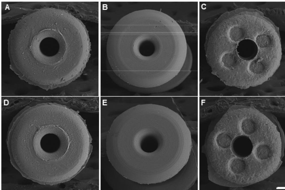
**Figure 3.** Image analyses of occluders. The top surface of the three types of unused (control) and with seven days in the presence of *S. aureus* (experimental) occluders were imaged using scanning electron microscopy (SEM). (A) Control Delta<sup>R</sup>; (B) Control Odyssey<sup>R</sup>; (C) Control Alphamed<sup>R</sup>; (D) Experimental Delta<sup>R</sup>; (E) Experimental Odyssey<sup>R</sup> and (F) Experimental Alphamed<sup>R</sup>. Scale bar = 100  $\mu\text{m}$ .
