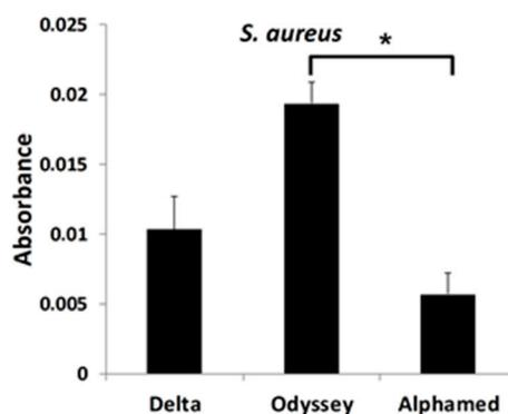
**Figure 2.** Quantitative measurements of bacterial growth on occluders. Occluders were placed individually in growing *S. aureus* for seven days. The presence of bacteria on occluders was determined by staining and elution with crystal violet. Absorbance of the eluted crystal violet was measured at an OD of 600 nm. \*  $p < 0.05$ .
